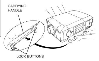
Pull up lock buttons to release lock.
